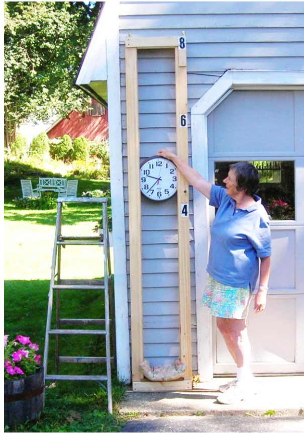
Figure 5 – Wall Clock Ready to Drop from 4 Feet in Guide Frame
